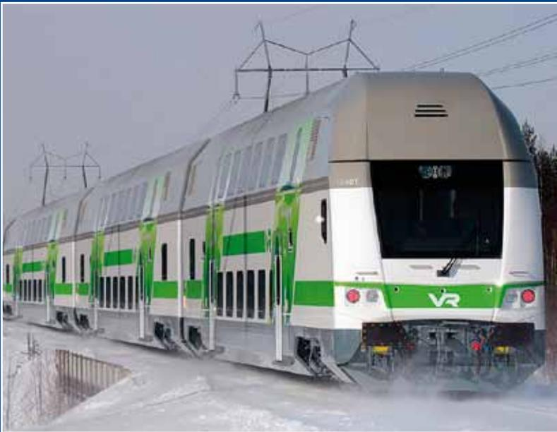
All double deck coaches are designed for a maximum speed of 200 km/h. The pressure-tight bodyshell is well insulated against sound and protects against traffic noise and pressure shocks, and is also safe in case of accidents.
